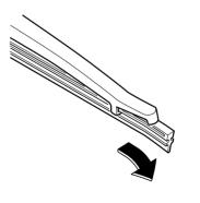
3. Remove the metal stiffeners from each blade rubber and install them in the new blade.
